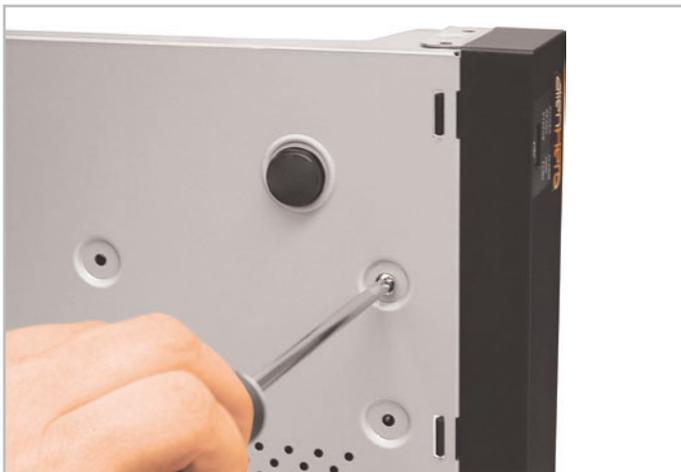
Screw through the four holes in the base of the DVR, and into the four fixing holes in the bottom of the hard drive shown on page 1. (Screws supplied with hard drive.)
