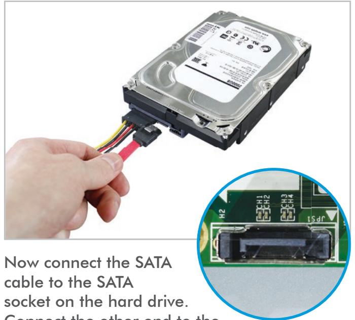
Now connect the SATA cable to the SATA socket on the hard drive. Connect the other end to the SATA socket on the PCB.
