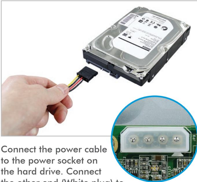
Connect the power cable to the power socket on the hard drive. Connect the other end (White plug) to the power socket on the PCB.
